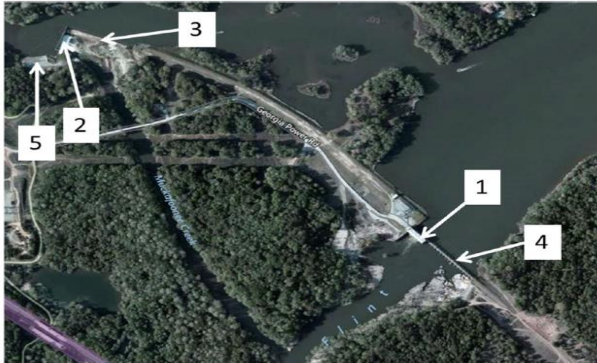
Figure 1: Flint River Project flow release mechanisms (listed in order of activation): 1) Powerhouse; 2) Muckafoonee Creek Dam spillway gates; 3) Muckafoonee Creek Dam free crest spillway; 4) Flint River Dam spillway gates 5) Emergency spillway
